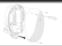
2 Disconnect pump motor cable. Remove pump assembly from the back plate to access the fixing holes.
